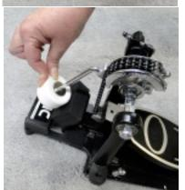
Loosely attach the eKIC onto the pedal and make sure that the beater is center on the pad before tightening any screws (beater OR eKIC)
